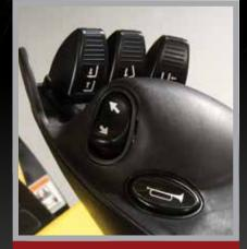
TouchPoint mini-levers with seatside direction control and auxiliary horn button
