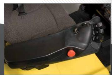
Electro-hydraulic controls with TouchPoint mini-levers
