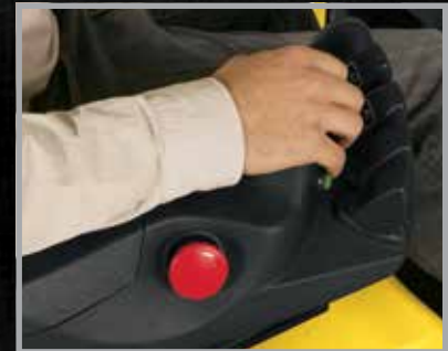
Electro-hydraulic controls with TouchPoint mini-levers
