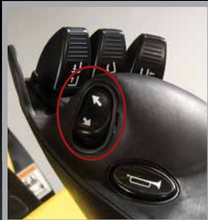
Electro-hydraulic controls with TouchPoint mini-levers
