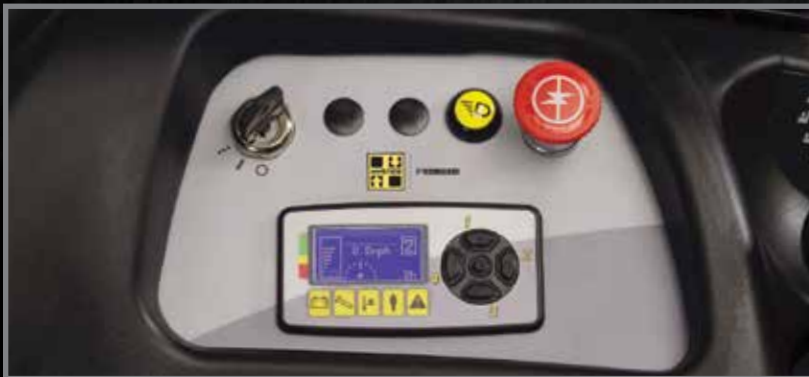
Hyster® i 3 Technology™ integrates commonality among Hyster warehouse products and simplifies the way in which operators and technicians alike handle and service the truck. This technology allows operator input to optimize performance to suit operator skill level. It also provides setup and diagnostic menus for service technicians.
