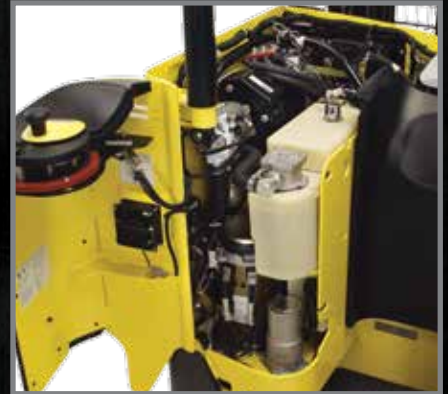
Uncluttered access to motor and controllers
