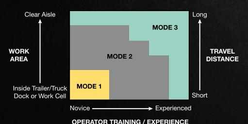
**Mode 1** – new operator, inside trailer, short distances, or for improved battery life
