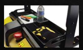
The W45Z<sup>+10</sup> with factory installed batteries includes an operator convenience tray with large storage area for stowing clipboards, pens, pencils and other items. Units equipped with a 9" battery box have several convenience tray options. (9" battery box option shown)
