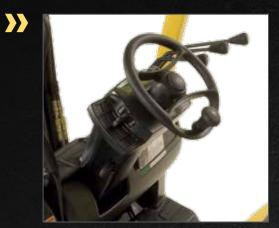
The 12-inch steering wheel rests on a tilting steer column, offering infinite adjustments and comfort.
