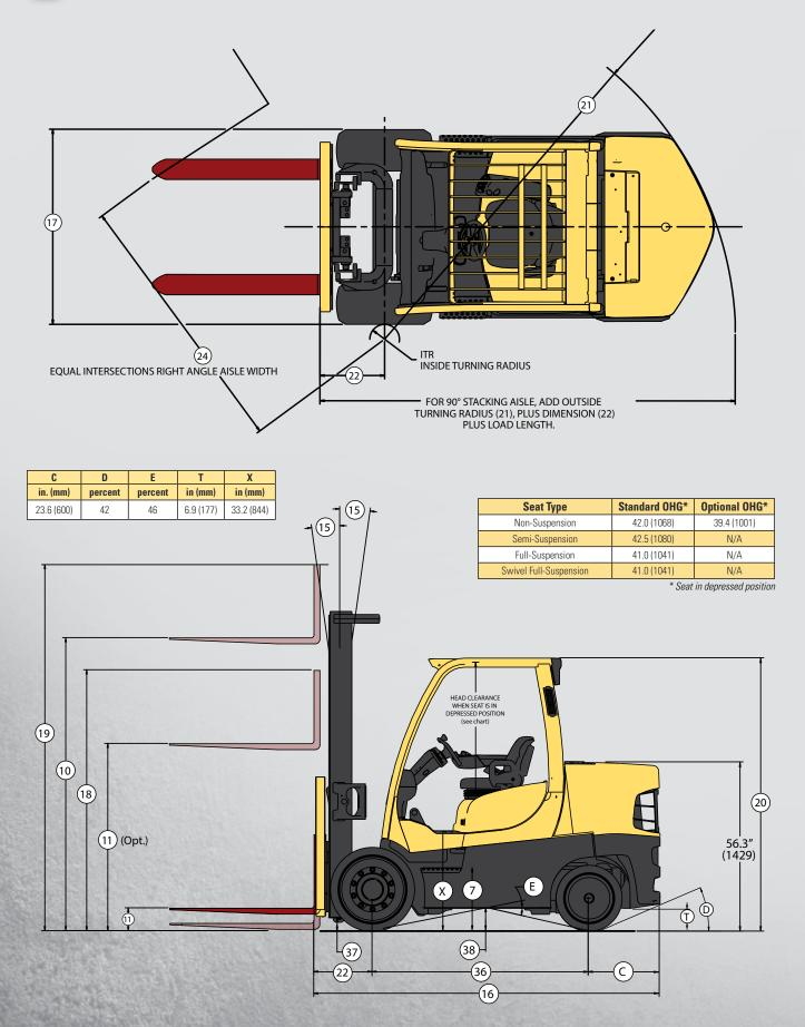
Circled dimensions correspond to the line numbers on the tabulated chart inside the Technical Guide. Dimensions are in inches (millimeters).
