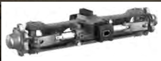
The steer axle assembly is made of cast ductile iron. Some competitors use welded plate structures that can suffer from cracks or deformation from shock loading, or steel plate structures that can bend.
