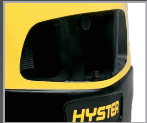
Counterweight tunnel design improves airflow
