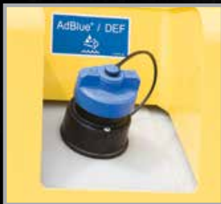
Diesel Exhaust Fluid (DEF) tank.
