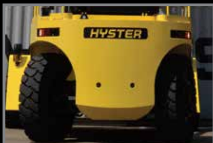
Rear sloping counterweight design.
