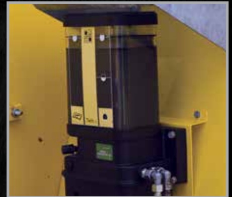
Optional automatic greasing system.
