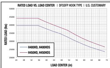
Model H400HDS: 40,000 lbs. at 36" (18,144 kg at 914mm) load center Model H450HDS: 45,000 lbs. at 36" (20,412 kg at 914mm) load center Model H400HD: 40,000 lbs. at 36" (18,144 kg at 914mm) load center Model H450HD: 45,000 lbs. at 36" (20,412 kg at 914mm) load center
