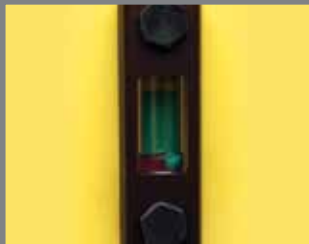
Hydraulic site glass located externally on the truck for clear/instant visibility of oil levels.
