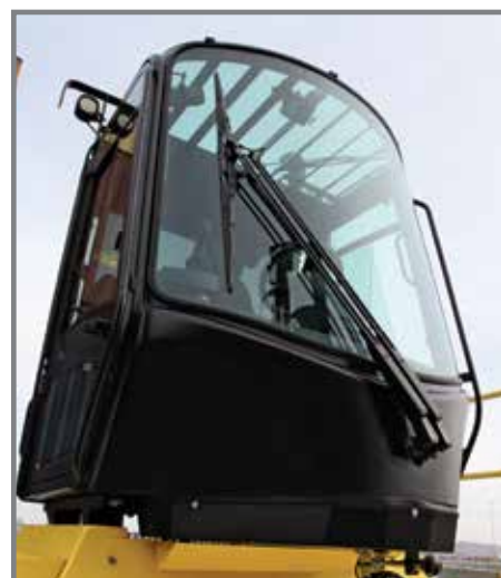
The ComforCab II offers large windows fitted with tempered safety glass, with excellent all-around visibility.
