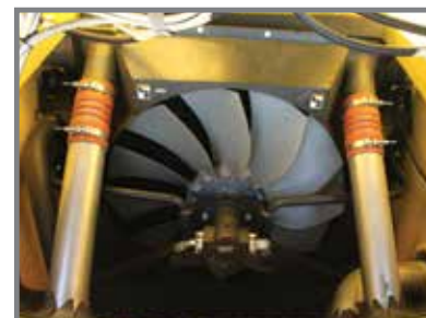
Puller fan draws cool and clean air.
