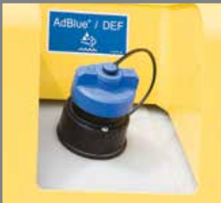
Diesel Exhaust Fluid (DEF) tank.
